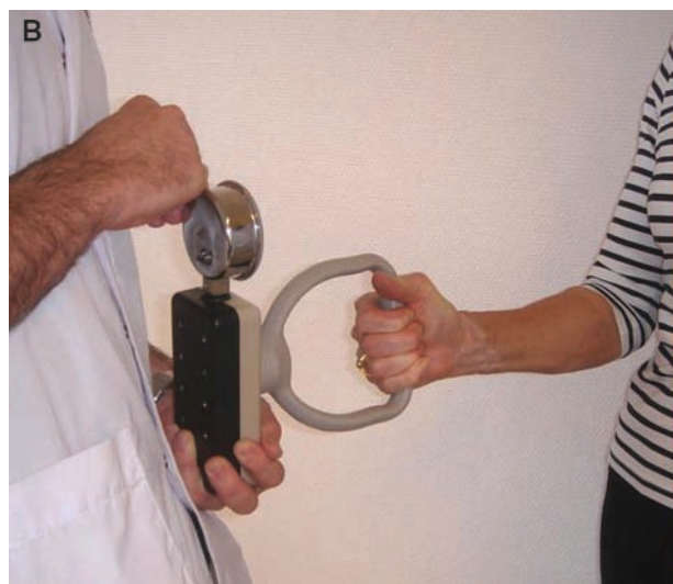
Figure 3. Mechanical dynamometers were used to measure strengths in elbow flexion (A) and forearm supination (B).
